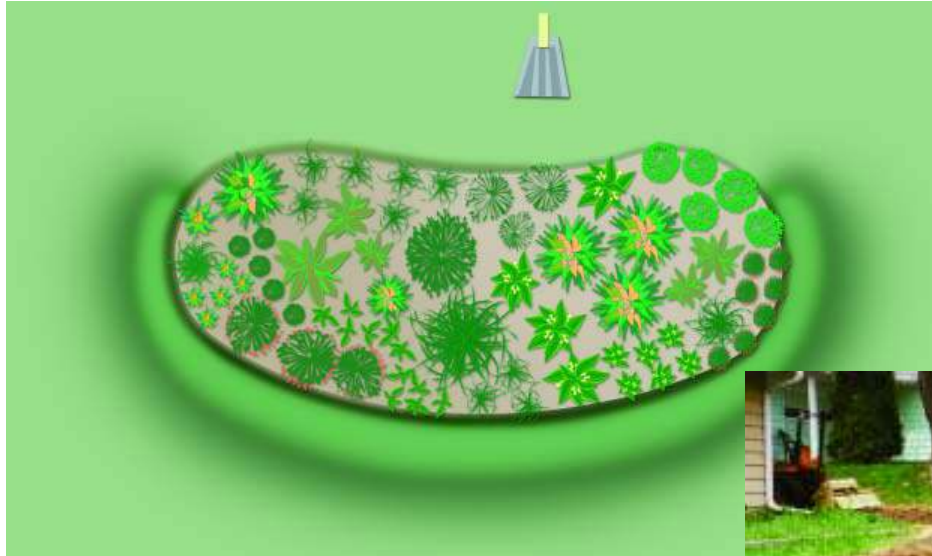
Figure 5 - The top of the downhill part of the berm should come up to the same elevation as the entry to the rain garden at the uphill end.
