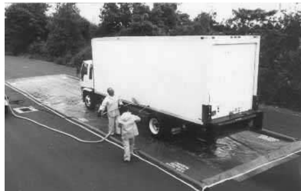
Portable Plastic Containment System (For Car Washing)
